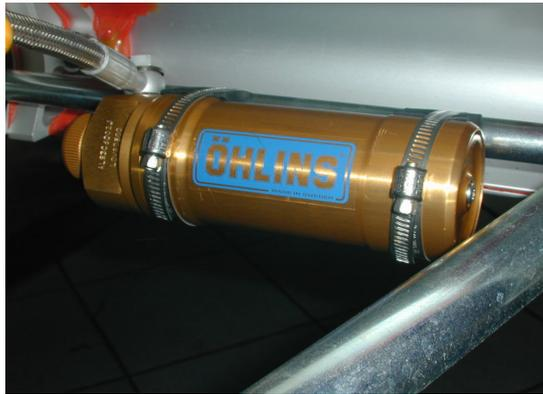
4. Fitting the Rear Canister – The Rear Canisters are Mounted in the same manner as the Front Canisters however these are mounted to the Rear Main Roll Hoop Stays as illustrated. On the Exige this will require fettling of the ABS Cover Panel, as illustrated below.
