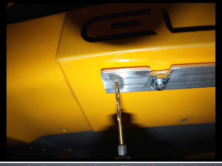
Place the center bracket under the clam shell in position. Notice the bolt in the bracket. The ends of the bolts are used to locate the bracket on the clam shell using the holes you drilled using the splitter as a template. Either hold or tape the bracket in place and drill pilot holes using the bracket as a template. Use a small drill bit smaller than 1/8" or you will remove the threads in the bracket.
