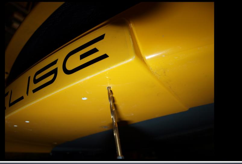
Enlarge the 6 pilot holes for the 3 brackets with a / " drill bit.
