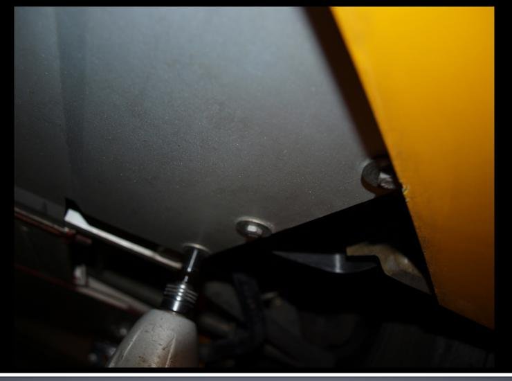
Remove the 3 bolts on both sides of the under tray.
