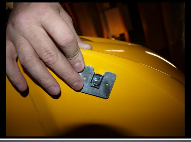
Using the same process as the center bracket repeat the process on the side brackets using the bolts to locate them on the clam shell and drill the 2 pilot holes for each bracket. Line the bracket up as in the picture with one edge parallel to the lip of the clam shell. This ensures that the bracket sits flat and does not end up being wedged along the inside lip of the clam shell.
