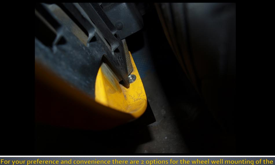
front splitter. The picture above shows the washer and lock nut being used. If you plan on removing/replacing the front splitter on a semi-regular basis you may want to make a small notch in the clam shell and use the u-nuts which are included in the kit. The notch will be the same as the notches in the aluminum brackets which simply let the u-nuts line up with the holes.
