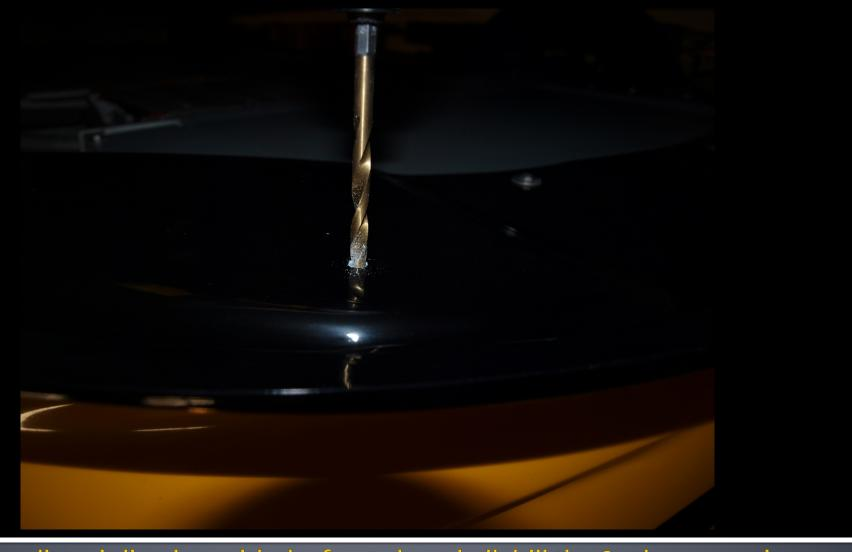
After the splitter is lined up with the front clam shell drill the 6 other mounting holes through the front clam shell using the splitter as your template being careful not to drill too far into the clam shell. You only want to drill through the fiberglass shell. The front splitter is pre-drilled with the size and locations of the holes. After the holes are drilled remove the splitter and set aside.
