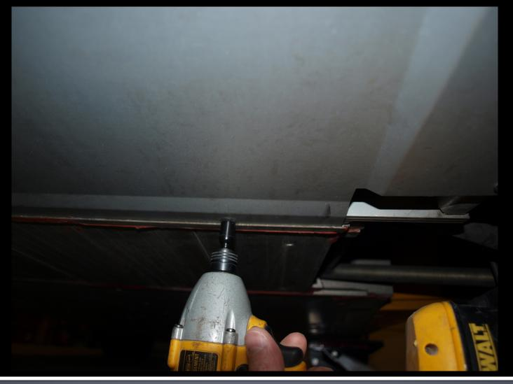
Remove the 3 bolts holding the rear edge of the under tray.
