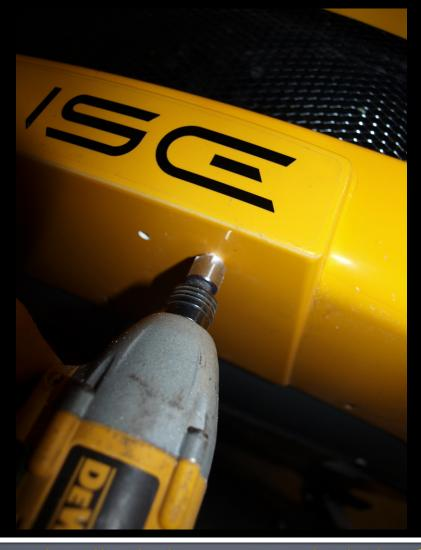
Use a counter sink bit on the pilot holes to taper the holes for the flat head bracket screws. Test fit the screws and taper the holes until the screws are flush. Take many quick passes with the bit rather than trying to get it in one or two passes. If you have never used a counter sink bit before practice on a piece of scrap wood or plastic to get some practice.
