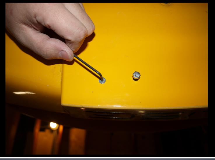
Place the center bracket inside the clam shell so it sits flat and line up the holes. Partially insert the 2 mounting screws to hold it in position and insert the 2 small flat head screws and tighten. Remove the 2 mounting bolts and set aside. Follow the same process for the side brackets. All 6 of the flat head screws should now be tight and flush and the 3 brackets in place.
