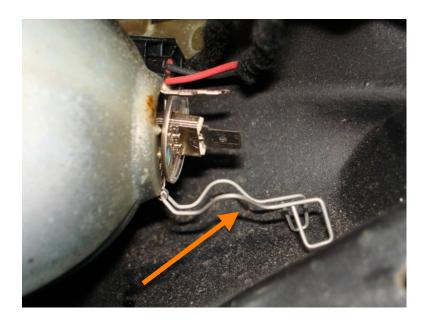
7. Carefully remove the bulb and replace with new one. Line up two lumps on the bulb fixing with the housing.
