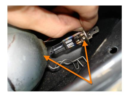
8. Reattach the metal clips and both cables, clean the seal and replace the headlight cover unit.
