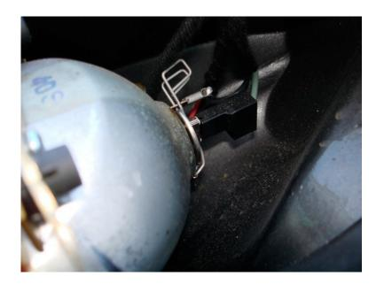
5. Remove the yellow coloured cable and the smaller black cable and push clear of the housing.
