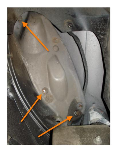
3. Once the three screws have been removed, you can slide out the lamp cover, being careful not to catch either of the lamp domes.
