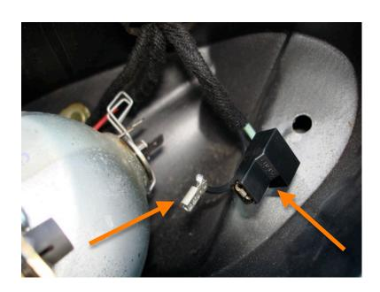
6. Unhook the two sliver clips holding the bulb in place.
