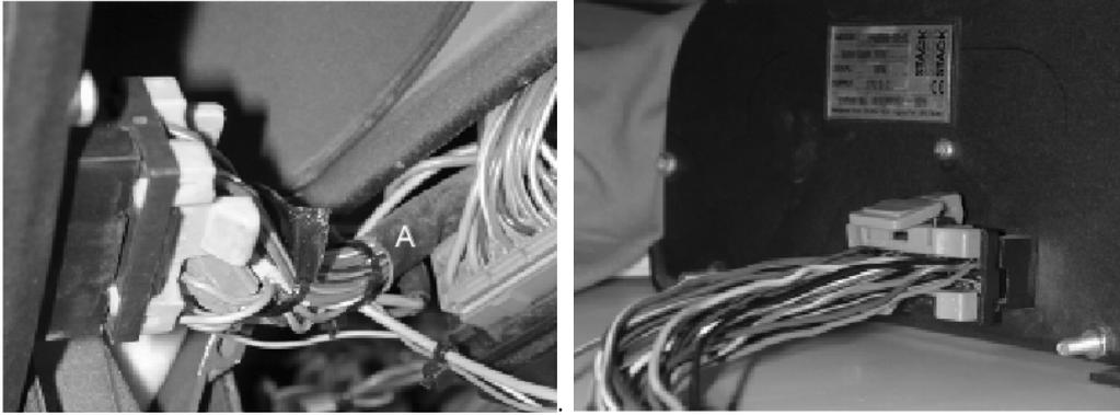
Some cars have the cable loom very close to the connector of the Instrument pack. You will need as much space as possible so if needed, cut the black tube which is pulled over the cable loom. Use the scissors, but be careful not to cut into wires!
