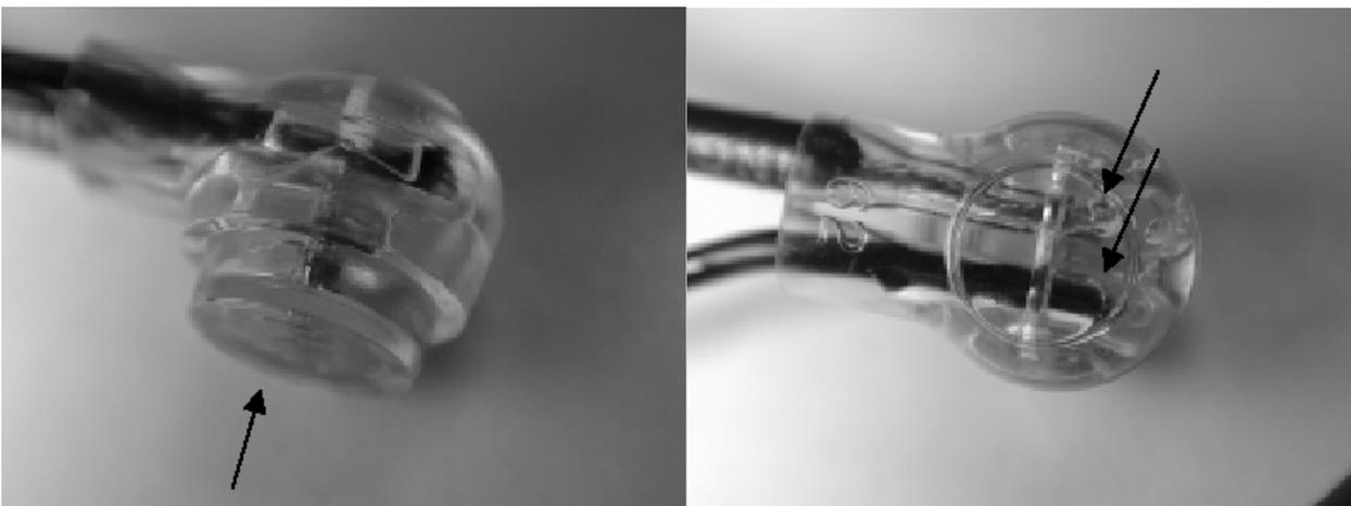
There are three transparent connectors in the package; these are meant to connect the wires of the switch to the fan controller. Please have a close look at the pictures to see
