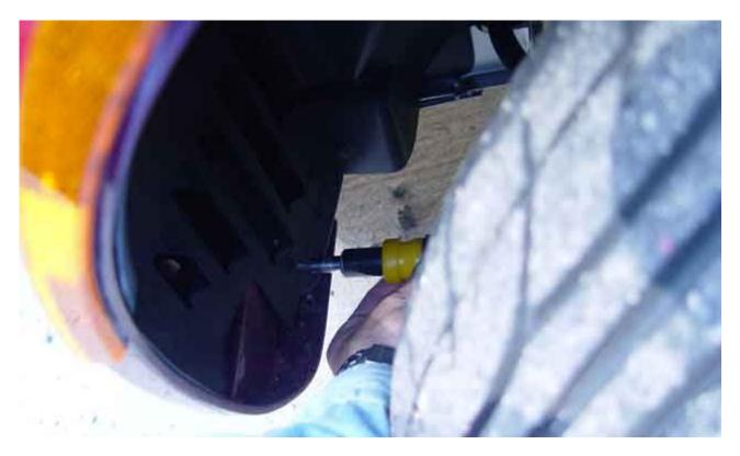
The metal screw is located high inside the wheel well. The picture below shows its location.
