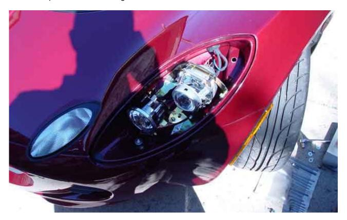
If you have small fingers it might be possible to remove the bulb without removing the entire headlight assembly. I however chose to remove the whole assemble so that I could see exactly how the bulbs are secured.
