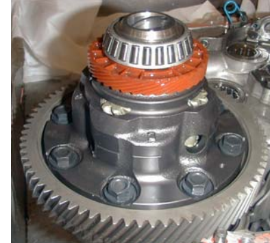
LSD unit contained within gearbox
