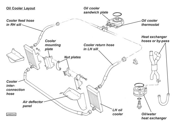
Each cooler is secured by a two stud bracket to the side of the crash structure, and positioned immediately ahead of the engine radiator mounting panel side extensions, which incorporate airflow apertures and additional deflector panels on their front surfaces. Louvres in the wheelarch liner front sections allow air to exhaust from the coolers into the wheelarches.
