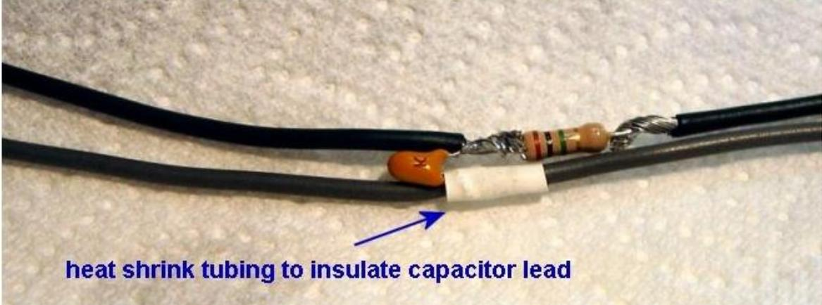
heat shrink tubing to insulate capacitor lead
